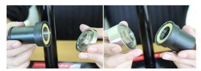
Step 2. Place both side tightly to the frame, and tighten the screw to install the bearing set into the frame.
