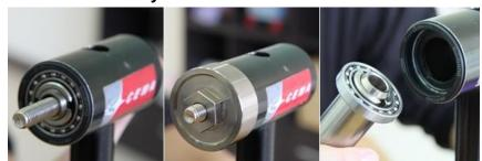
Step 4. CEMA Bearing Kit. Place CEMA bearing (SRC-BB-S003 / SRC-BB-S005) onto adapter and fit bearing cup (OD25mm).
