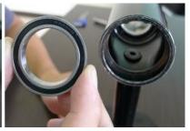
Step 3. CEMA Bearing Kit. Place CEMA bearing (SRC-BB-BC30 / SRC-BB-BS30) onto the adapter (30mm) and fit the frame, place the adapter on another side to place correctly.
