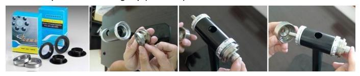
Step 5. Tighten screw to fit bearing and then replace caps.
