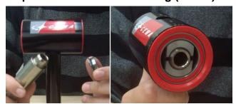
Step 4. Insert screw add spacer (PF30 / 386) and thread on bearing cup into the tube then tighten the external bearing cup.
