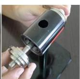
Step 4. Tighten cup and screw to fit bearing and then replace caps. Repeat the process for the other one.
