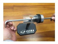
Step 4. Tighten the hex wrench and remove the hand adapter.
