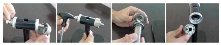
Step 4. CEMA Bearing Kit. Place CEMA bearing (SRC-BB-S003 / SRC-BB-S005) onto adapter and fit bearing cup (OD25mm).
