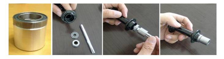
Step2. Insert threaded screw and external bearing adapter thread on tightening bars and tighten to fit bearings.
