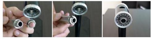
Step 3. Insert thread screw and fit bearing cup. Tighten screw to remove bearing.
