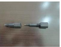
Step2. Push bearing puller into bearing and tighten.
