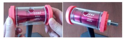
Step 3. Tighten up the bottom bracket to the bottom bracket shell until there is no gap between the bracket and the shell.
