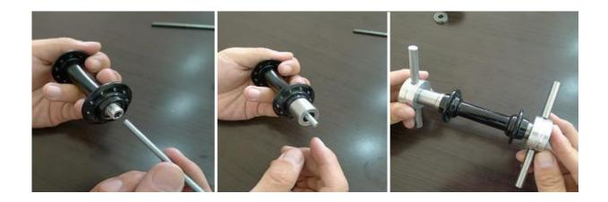
Step3. Insert one bearing onto axle and other bearing into HUB insert threaded screw and external bearing adapters and tightening bars, tighten to fit bearings.
