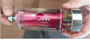
Step 3. Tighten the screw and remove the bearing.
