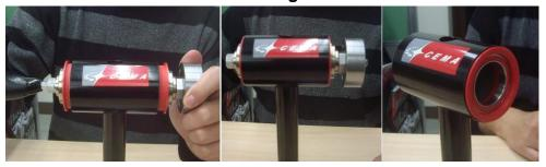
Step 3. Place the removal ring (30mm) onto the extractor tube and insert into BB.
