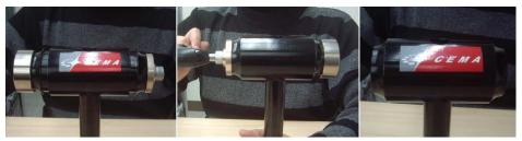
Step 3. Insert the extractor tube with the removal ring (30mm, PN: SRC-TT-B006C-09) through the frame to the bearing.
