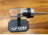
Step 3. Press-fit the thread screw and roll hex wrench while making sure that the rim of the hand adapter stays parallel to the rim of the external bearing cup.
