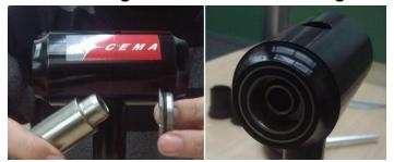
Step 4. Insert screw add spacer (PF30 / 386) and thread on bearing cup.
