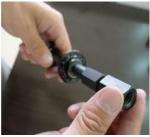
Step 3. Screw puller handle into bearing puller and slide handle weight sharply downwards to remove bearing.
