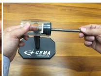
Step 2. Insert the thread screw into the spacer (BB86/PF30/386) and the external bearing cup. Then lock the external bearing cup.
