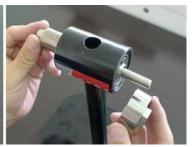
Step 2. Tighten the screw to remove the bearing, repeat process for the other one.
