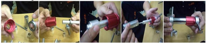
Step2. Use the same process to fit the second bearing.
