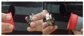
Step 2. Place both side tightly to the frame, fit the external bearing cup and tighten the screw to install the bearing set into the frame.
