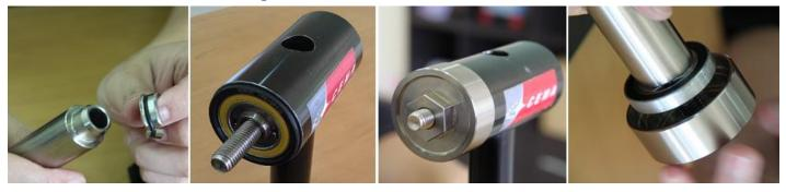
Step 3. CEMA Bearing Kit. Place the spacer first, CEMA bearing (SRC-BB-S004 / SRC-BB-S006) onto the adapter (22mm) and fit bearing cup.
