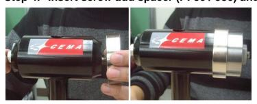
Step 5. Tighten the screw to remove the BB set. Repeat the same process for another one.
