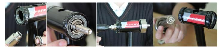
Step 3. CEMA Bearing Kit. Place the spacer first, CEMA bearing (SRC-BB-S004 / SRC-BB-S006) onto the adapter (22mm) and fit bearing cup.
