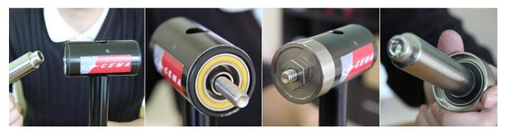
Step 2. Place the removal ring(24mm, PN: SRC-TT-B006C-08) then insert the extractor tube through the Drive side bearing, lock the external cup, and tighten the screw to remove the bearing.
